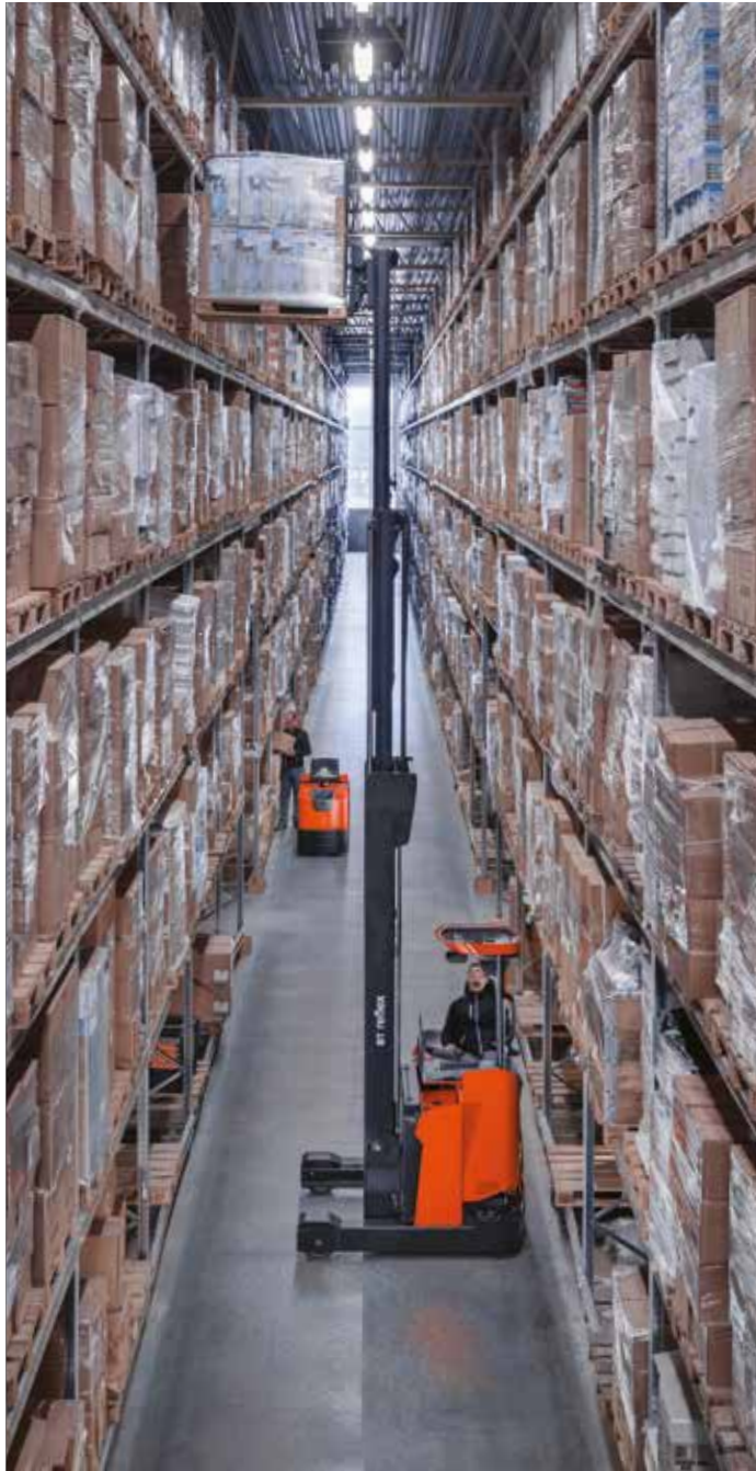
The open fork carriage with integrated side shift offers excellent visibility forward.
