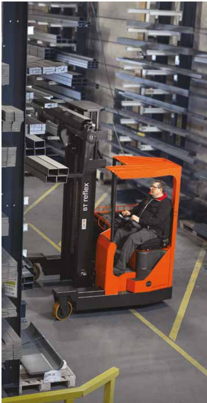
BT Reflex F-series' hydraulic fork spreader quickly adapts the truck to loads of different dimensions
